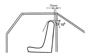
i) All seats are to be fitted with headrests to reduce the chance of neck injury in front and rear collisions.
